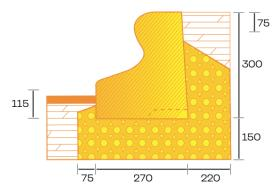
BS7263 (1994) Complies with all the relevant specifications Transverse strength specification exceeded by 70%
